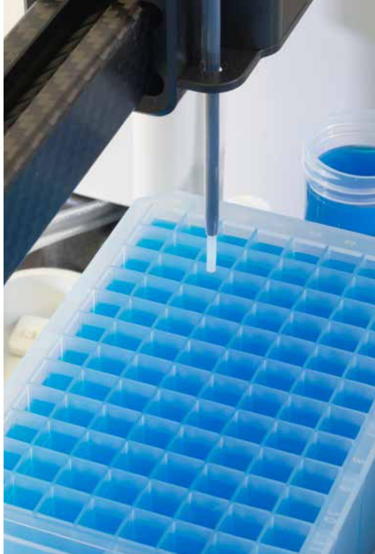
Close-up view of 0.9 mm ID sample probe with 96 well plates
