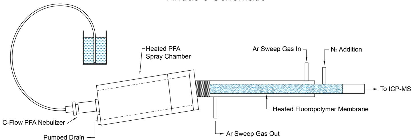
**Figure 1. Teledyne CETAC Aridus3 Schematic:** Aridus3 core components consist of a PFA nebulizer, a heated PFA spray chamber, and a heated fluoropolymer membrane desolvator; built-in mass flow controllers set the Ar sweep gas and N<sub>2</sub> addition gas flows.
