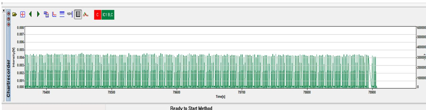
Figure 4. Scan of  $^{235}\text{U}^+$  Signal using Thermo Neptune MC-ICP-MS with Teledyne CETAC Aridus3 (beta-unit)
