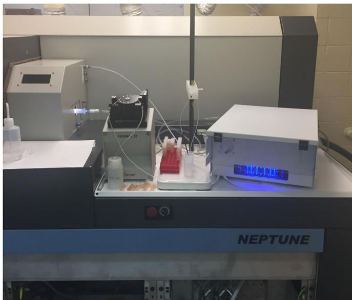
**Figure 2. ThermoFisher Scientific Neptune MC-ICP-MS & Teledyne CETAC Aridus3 (beta version, at far right with blue ready status light)**
