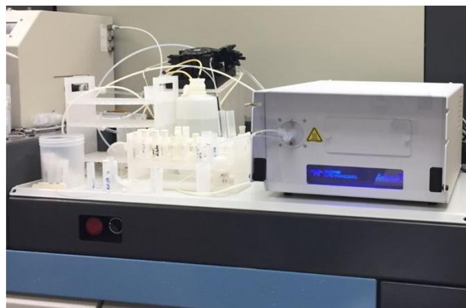
**Figure 2. ThermoFisher Neptune MC-ICP-MS & Teledyne CETAC Aridus3 Desolvating Nebulizer System**
