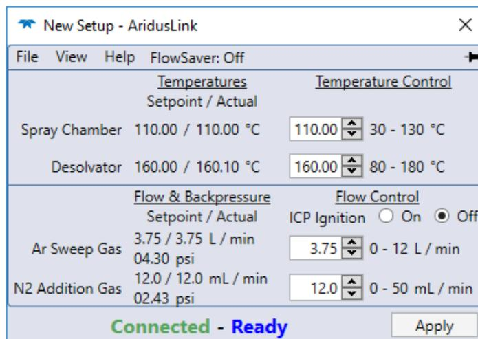
**Figure 4. AridusLink Software Control Screen**
