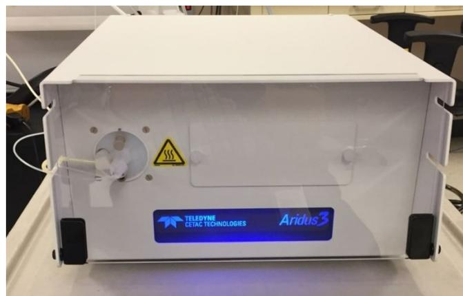
**Figure 1. Teledyne CETAC Aridus3 Desolvating Nebulizer System – Front View**
