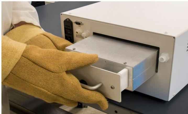
**Figure 3. Aridus3 Removable Membrane Oven Module**
