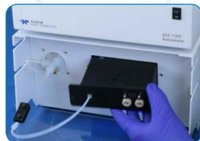
Installation of QuickWash Fast Washout Accessory for the Aridus3
