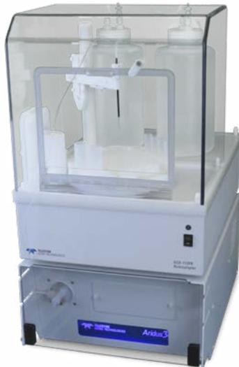
There are five standard positions for 20-mL PFA vials and nine standard positions for 4-mL PFA vials. Sample racks include 24, 48, and 96 position types for 0.5 mL to 2.0 mL sample volumes. Bel-Art half racks (30 and 42 position) for 7-mL and 14-mL samples are also available.
