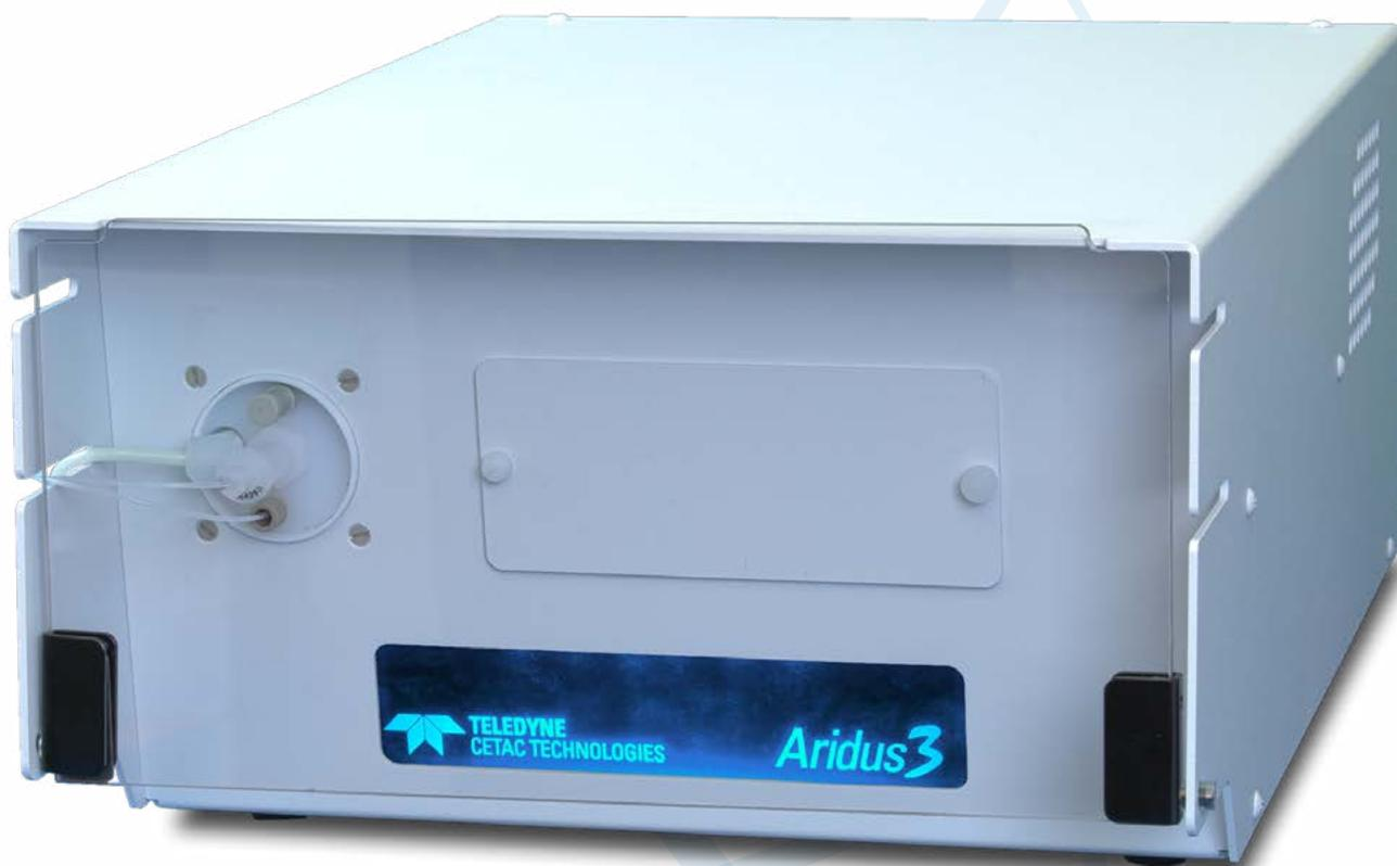
The Teledyne CETAC Aridus3 Desolvating Nebulizer System is a specialized liquid sample introduction accessory for inductively coupled plasma mass spectrometry (ICP-MS). The Aridus3 can enhance analyte sensitivity up to 10 times or more and can greatly reduce solvent-based interferences such as oxides and hydrides.
